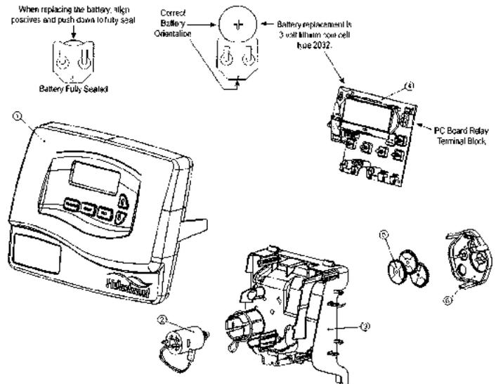
After completing any valve maintenance involving the drive assembly or the drive cap assembly and pistons, press and hold NEXT and REGEN buttons for 3 seconds or unplug power source jack from the printed circuit board (black wire) and plug back in. This resets the electronics and establishes the service piston position. The display should flash all wording, then flash the software version (ex: 214) and then reset the valve to the service position.
